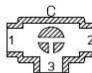
N.B. please choose the rest position of the ball when the SR actuator is used, paying attention to the fact that this actuator turns in an anti-clockwise direction, whenever supplied with air.
